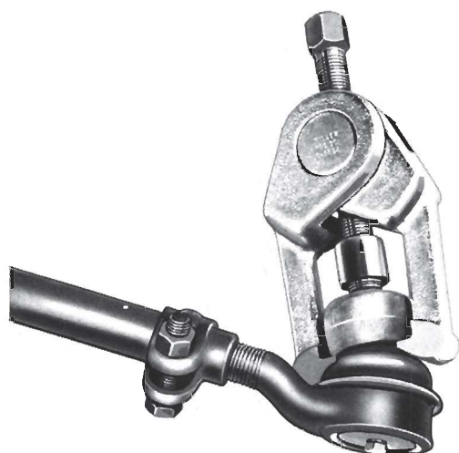
Fig. 9—Removing Tie Rod End Stud from Steering Knuckle Arm
