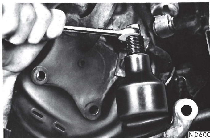
Fig. 16—Removing Lower Ball Joint Stud
